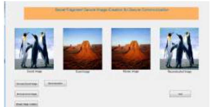
Fig 2: simulation results of Mosaic image constructed with selected target and secret image and secret image retrieved from the Mosaic image.
