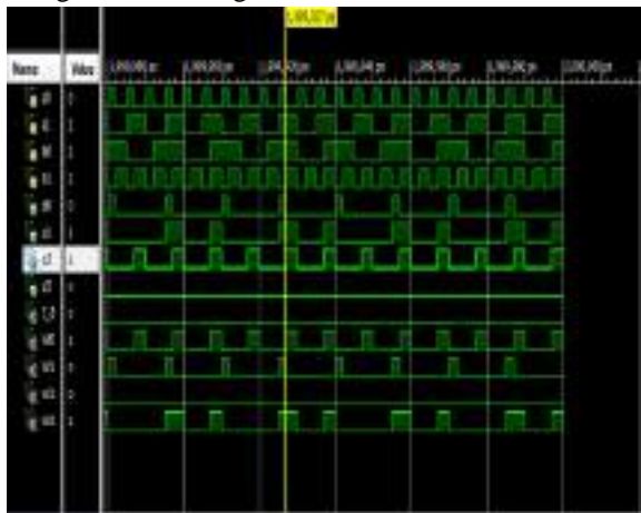
Fig.10: Simulation results for reversible 2*2 Vedic multiplier.
