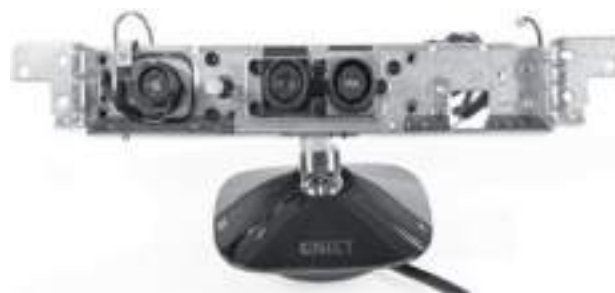
Figure 1 The infrared (IR) projector, IR camera, and RGB camera inside a Kinect sensor.
