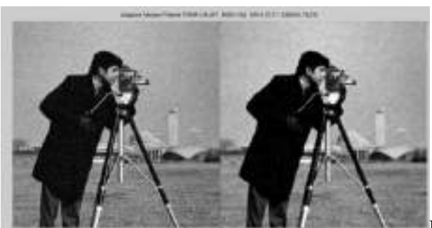
Figure 6 AWGN Noisy Image Vs Adaptive Median Filter output
