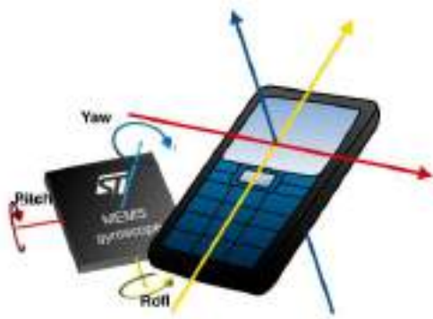
Fig 3: Gyroscope Three Axes on Smartphone's.
