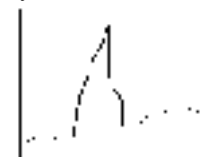
Fig-5 Spike fault
