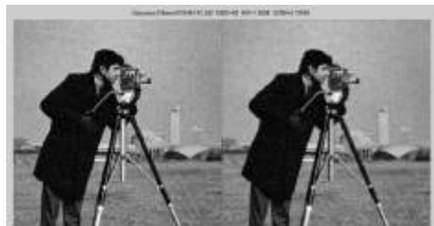
Figure 3 AWGN Noisy Image Vs Gaussian Filter output
