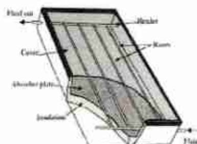
Fig. 1. Thermal model of the solar flat plate collector
